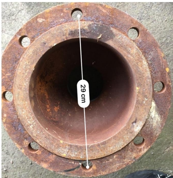
Flange 5. DN 200, 8 inch – 8 holes
